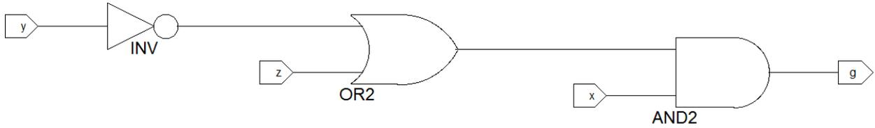
**Figure 3:** Function  $g(x, y, z)$  schematically implemented.
