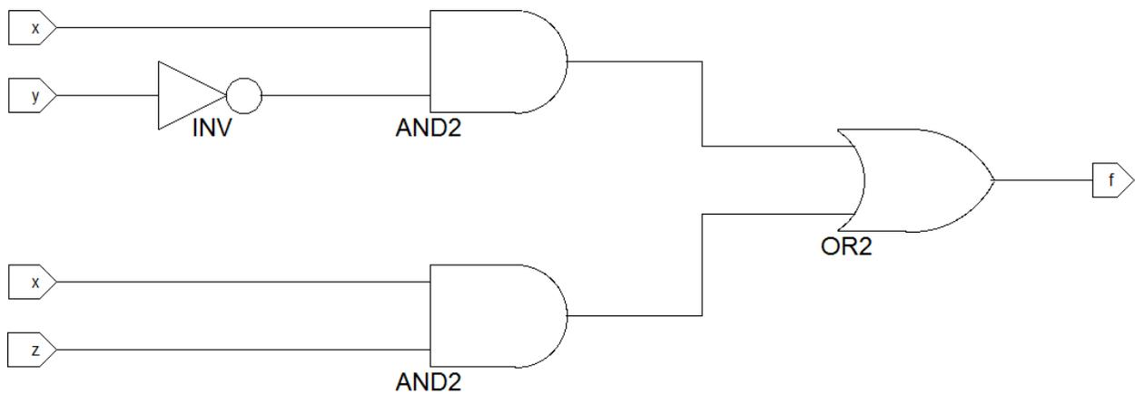
**Figure 1:** Function  $f(x, y, z)$  schematically implemented.
