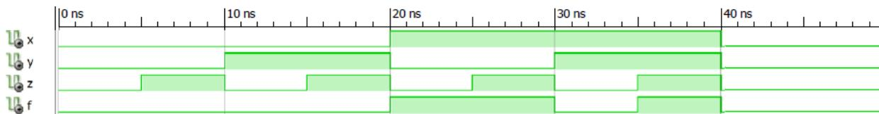
**Figure 2:** Output of the simulated circuit of function  $f(x, y, z)$ .
